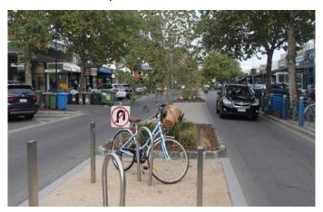
The above photo shows use of wide medians. In addition to providing a safe waiting spot between cross directional traffic, it allows bicycle parking, street trees, space for public seating and other features to enhance the surrounding area.
